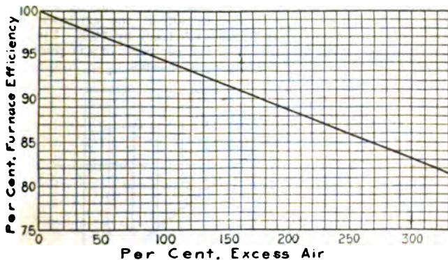
Fig. 3. Relation between furnace efficiency and excess air.
